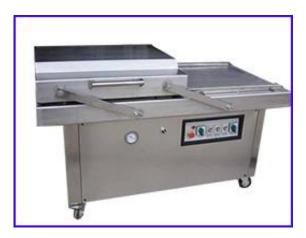
This process is preventing air penetrating into bags to keep potato chips fresh long time. It is applied in a small scale potato chips French fries making plant.
