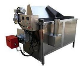
One of the most obvious advantages is LPG and gas is as the heating source, without heavy load power supply.
