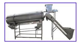
Continually Fries Drum Seasoning Machine is suitable for applying in an industry chips and fries production plant process.
