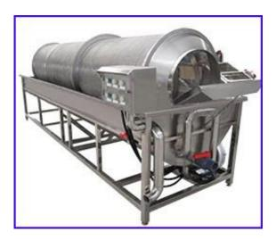
In an industry potato chips French fries making plant, due to the large final products capacity, potatoes should be have a preliminary washing before going to peeling process.
