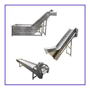
De-stoning Elevator is the first step machine for a large fries making process to deposit sand and soil from the potatoes.
