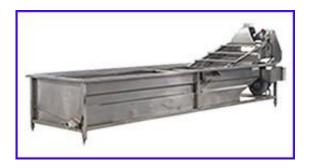
For the automatic frying or frozen chips process, the slices fall into a cold-water air bubble washing machine that removes the starch released when the potatoes are cut. Some manufacturers, who market their chips as natural, like banana and plantain chips, normally do not wash the starch off the potatoes.
