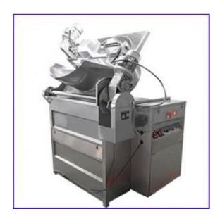
For small scale banana chips or plantain chips making process, it is a batch operation from slicing and frying. The small banana chips plantain chips fryer is recommended. This chips frying machine uses electricity as heating source with stirrer and automatic discharge operate. It is almost automatic instead of agitation by hand during frying.
